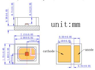
VD-0940P-050W-3A-3A0 (Channel array 1X1, Substrate CuAg, Package 2016)
