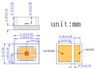
VD-0940P-025W-3A-3A0 (Channel array 1X1, Substrate CuAg, Package 2016)
