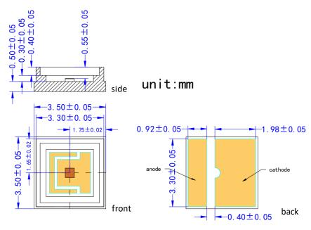
VD-0940C-070M-3C-2A0 with Substrate 3=Cu/Ag and Package C=3535 (unit: mm)
