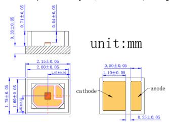
VD-0850P-025W-3A-3A0 (Channel array 1x1, Substrate CuAg, Package 2016)
