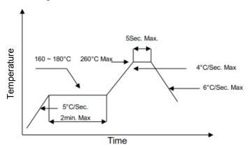
Note: Reflow soldering can be operated only one time. During the temperature ramp-up, no forces may be exerted on the LD which could deform or damage them. After soldering completed, please also do not process until the product temperature ramp down to room temperature.
