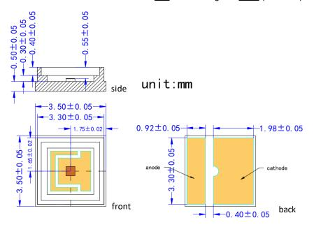
VD-0850I-004W-1F-2A0 with Substrate 1=AIN and Package F=7070 (unit: mm)
