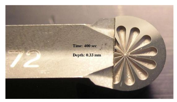
3D laser milling on a chip breaker
