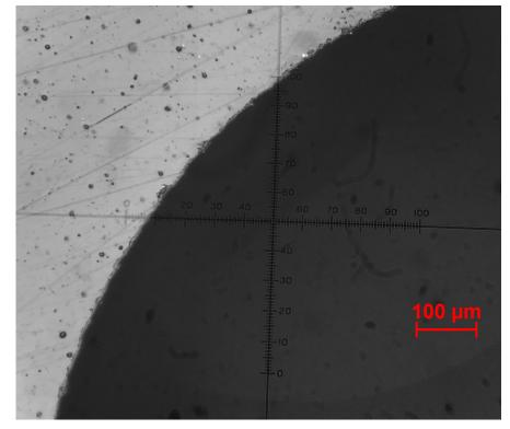
2 mm diameter hole cut – laser exit side
