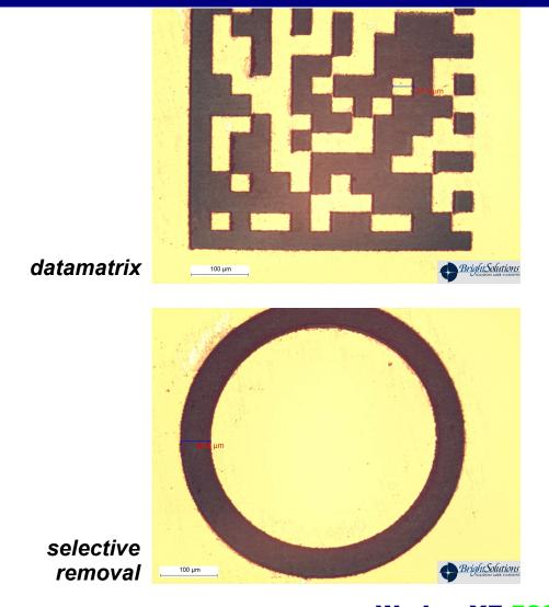
Precision micro-marking on polymeric materials
