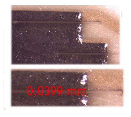
*laser trimming for accurate control of electric resistance in circuit components*
