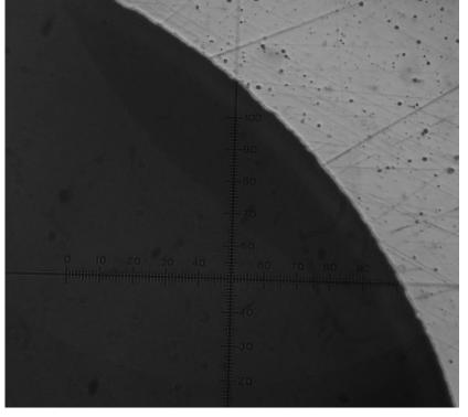
2 mm diameter hole cut – laser entrance side
