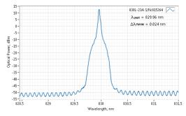
Typical spectrum of 0830 nm diode laser. Measured with 20 pm resolution.
