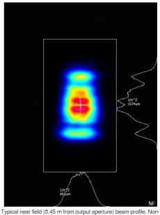
circularized beam of a 0450 nm direct diode laser.
