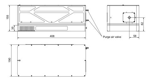
High average power version. Q-SHIFT laser head dimensions (in mm)
