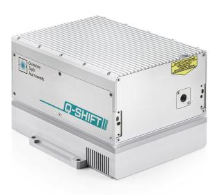
Q-SHIFT is family of Q-switched lasers with build-in nonlinear wavelength conversion stage that allows to produce wavelengths that are not accessible with conventional solid-state laser sources. As pump sources our Nd:YAG or Nd:YLF lasers of Q2 or Q2HE series are used.
