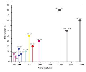
High peak intensity pulses at visible wavelengths (blue, yellow and red) are provided when Q-SHIFT laser is combined with our attachable SHG or stand-alone H-SMART harmonic generator.
