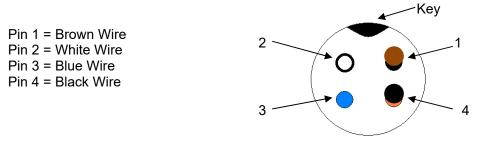
Diagram shows the connector mounted to the module
