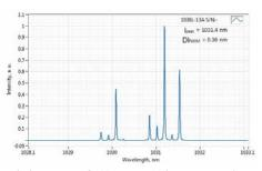
Typical spectrum of 1030 nm DPSS laser. Measured with 20 pm resolution.
