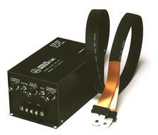
The **779A** Series laser diode drivers are designed to power high current laser diodes for applications such as laser pumping and illumination. A pulse generator with adjustable amplitude, width, PRF and current limiting is included. A CW enable and opto-isolated pulse input also provide for remote control. The 779A Series provides negative current for grounded anode emitters using a closed-loop current source.
